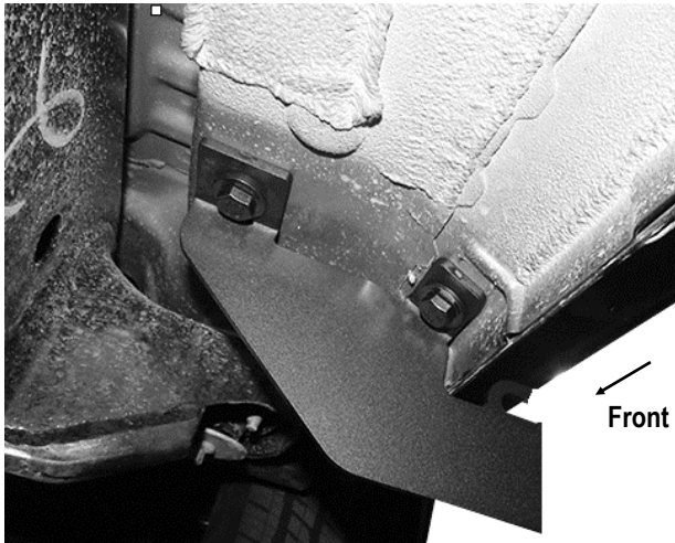
(Fig 3) Passenger Front Mounting Bracket (PFM) Installed
