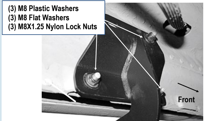
(Fig 5) Driver Rear Mounting Bracket Installed
