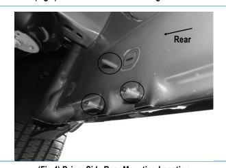
(Fig 4) Driver Side Rear Mounting Location
