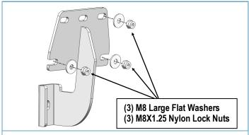
(Fig 2) Driver Front Mounting Bracket Installation
