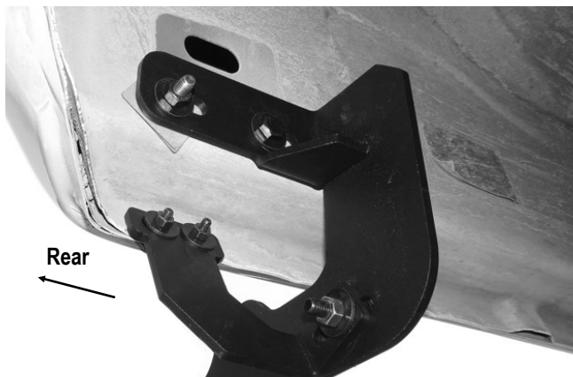
(Fig 12B) Driver Rear Brackets installed
