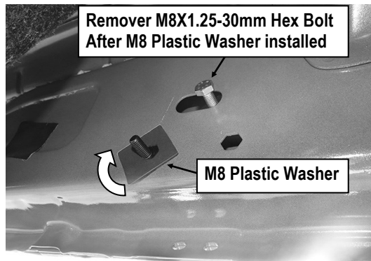
(Fig 5) Thread Plastic Washer Onto the Welded Bolt on M8 Bolt/Nut Plate To Hold Bolt/Nut Plate In Position. IMPORTANT: Do Not Remove The Hex Bolt Until The M8 Plastic Washer Has Been Threaded Onto the Welded Bolt.
