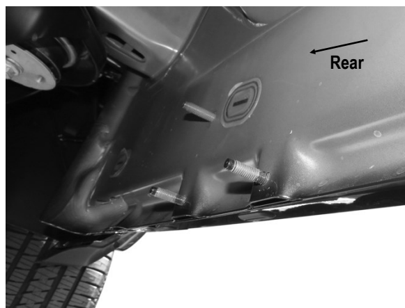
(Fig 4) Driver Rear Mounting Bracket Location Pictured
