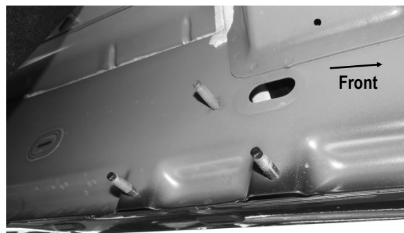
(Fig 3) Driver Center Mounting Bracket Location Pictured
