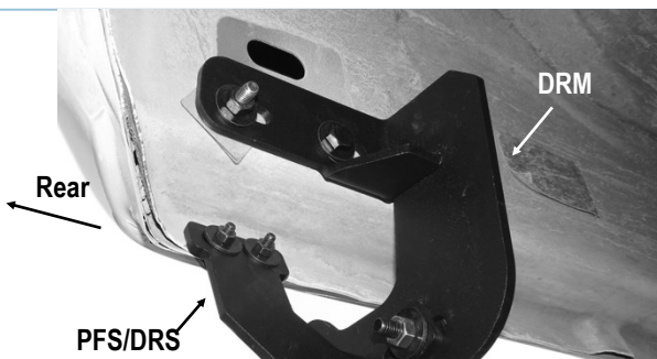
(Fig 14) Driver Rear Brackets installed
