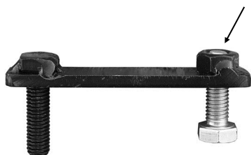
(Fig 3) Thread (1) M8X1.25-30mm Hex Bolt into the nut on the plate. Stop when bolt reaches end of nut as pictured)
