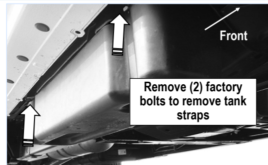
(Fig 12) 07-16 Passenger side DEF tank and cover
