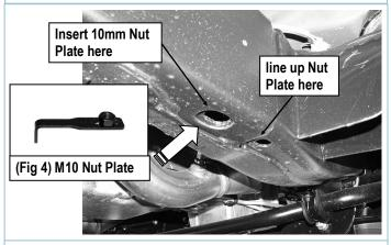
(Fig 3) Passenger Side Front Support Bracket Mounting Location
