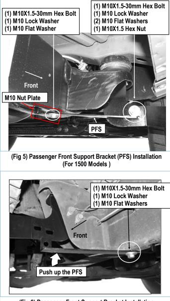
(Fig 6) Passenger Front Support Bracket Installation (For Up to 2007 2500/3500 Models)
