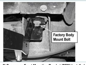
(Fig 2) Passenger Front Mounting Bracket (PFM) Installed
