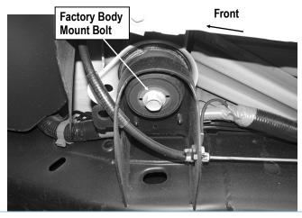
(Fig 1) Passenger Side Front Mounting Location
