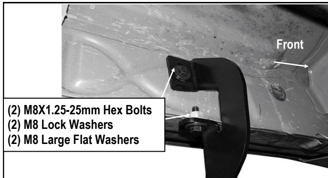
(Fig 6) Driver Side Front Bracket Installed
