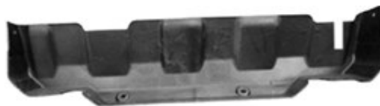
(Fig 15) 2017-Up Passenger Side DEF Cover Marked For Trimming
