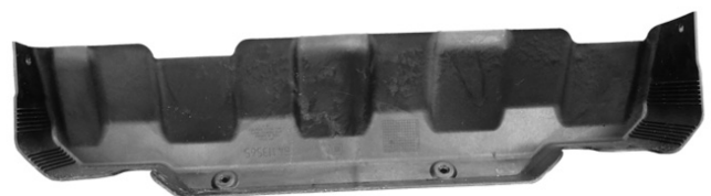
(Fig 9B) 17-on Passenger side DEF cover removed
