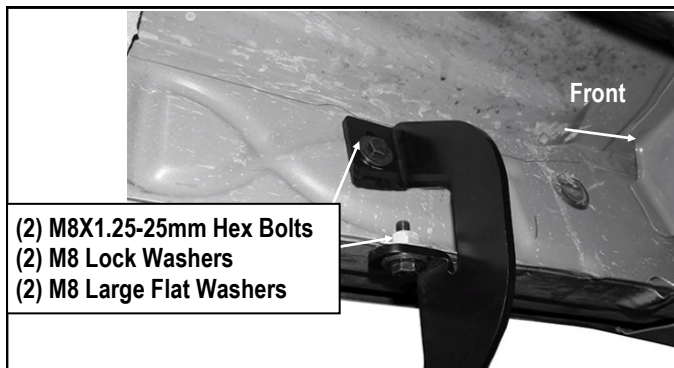
(Fig 6) Driver Side Front Bracket Installed
