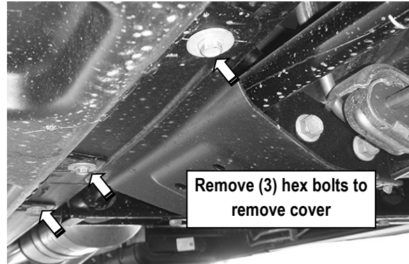
(Fig 11) 07-16 Passenger Side Front Pictured with DEF Tank Cover.
