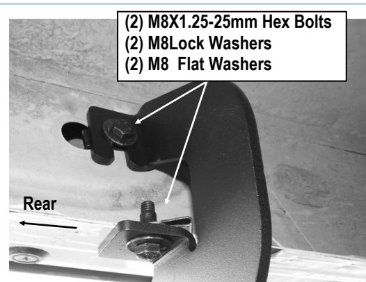
(Fig 9) Driver Center Bracket Installed
