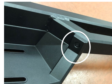
M6X1-20 Flat Sunk Head Bolt Location
