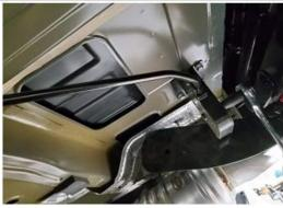
Lower the exhaust by removing the three rearmost rubber holders from the exhaust hangers. Use a stand to support the exhaust and prevent any damage. The exhaust will be reinstalled in Step 3.
