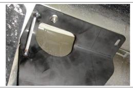
Mark and drill the forward most holes in the frame rail using the trailer hitch as your guide. Fishwire a M12 carriage bolt and square-hole spacer into each drilled hole and secure the hitch with a hex flange nut.
