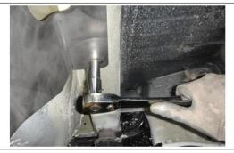
Torque M12 Carriage Bolt to 58 ft-lbs. Reinstall the heat shield, raise the exhaust back into position and reinstall the rubber isolaters.
