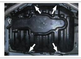
Remove existing M14 bolts. There will be (4) or (6) bolts depending on vehicle model. Retain (4) bolts for hitch installation. Keep the remaining bolts (if any).
