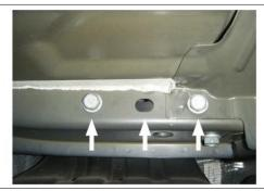
4 Raise the trailer hitch into position and reinstall (4) M14 bolts.
