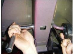
Reinstall heat shield, fasteners, and exhaust removed in steps 1 & 2. Installation Complete.
