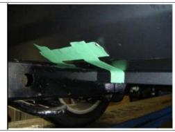
Push hitch in rearmost position and secure hitch to the frame with (4) flange nuts. Torque all M12 fasteners to 86 ft-lbs.
