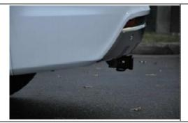
\*\*\*Periodically Check The Receiver Hitch To Ensure That All Fasteners \*\*\*
