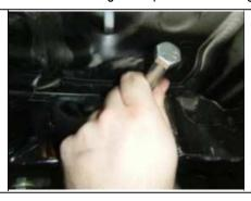
6 Torque M10 hardware to 47 lb-ft. Raise exhaust and spare tire back into position.
