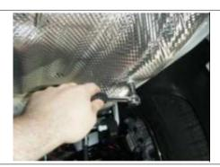
Raise hitch into position by raising passenger side of hitch over exhaust and secure into position with supplied M10 Hex bolts and M10 conical washers, as shown. NOTE: If the vehicle fascia prevents the hitch from being raised completely into position see trim diagram on page 1.
