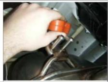
Remove heat shield by removing (3) nuts and (1) screw. Trim heat shield to allow hitch side plate to rest against vehicle frame rail. The area trimmed off will remove approximately 8 inches of the heat shield that was along the inside of the frame rail.
