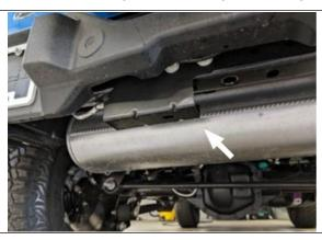
3 Tighten all fasteners. Torque M12 hardware to 86 ft-lbs.
