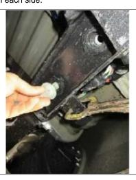
2 Raise hitch and into position, use existing hardware removed in step 1 to secure hitch and assembly to vehicle.
