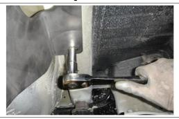
Torque all M12 Fasteners to 86 lb-ft. Reinstall the heat shield, raise the exhaust back into position and reinstall the rubber isolaters.
