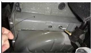
Slide the hitch in from the rear passenger side of the vehicle over the exhaust and into position. **Note:** Feed the fishwires through the mounting holes while raising the hitch.
