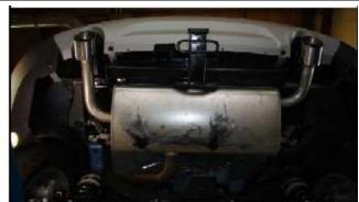
Torque all M12 hardware to 86 ft-lbs. Torque all M8 hardware to 23 ft-lbs. Re-attach rubber isolator removed in Step 1. Installation Complete.
