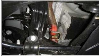
Remove the (1) fastener securing the heat shield to the bottom of the driver side frame rail. Trim the portion of the heat shield covering the mounting areas of the driver and passenger side frame rails, see trim diagram. After trimming reattach the heat shield to the bottom of the driver side.
