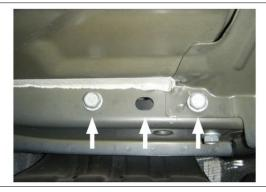
Raise the trailer hitch into position and reinstall (4) M14 bolts.
