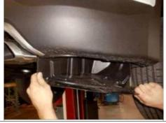
Raise hitch into position and secure to the existing weldnuts with M10-1.25 x 25mm bolts and conical toothed washers.
