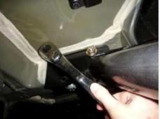
Torque all M12 hardware to 86 ft-lbs. Torque all M10 hardware to 48 ft-lbs. Raise exhaust and spare tire back into position. Reinstall passenger side and driver side under body panels removed in Step (3).
