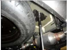
2 Lower exhaust by removing (3) rubber isolators.
