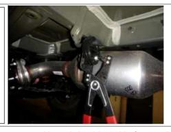
Remove the plastic under body panel from the passenger side and the driver side frame rails. Remove (3) fascia screws from the passenger side and (4) from the driver side. Carefully pull down and set aside.
