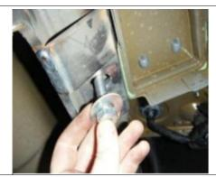
6 Torque M12 Carriage bolt to 58 lb-ft and other M12 hardware to 86 lb-ft. Raise exhaust back into position.
