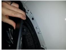
Gently unclip (1) reflector on each side of rear fascia to access and remove (1) fastener on each side using 8mm socket.
