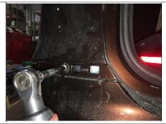
Remove (6) screws located on bottom of bumber fascia, if present unplug electrical harness.
