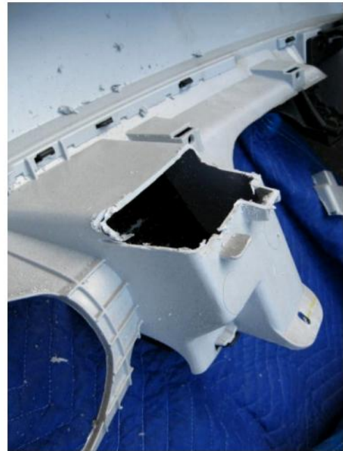
USING A ROTARY OR EQUIVALENT CUTTING TOOL, TRIM BUMPER FASCIA AS SHOWN TO THE RIGHT.
