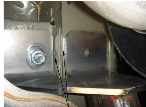
SIDE PLATE WILL STRADDLE THE SEAM BETWEEN THE FRAME RAIL AND THE BUMPER BEAM
