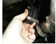
Remove (2) rubber isolators from muffler. Remove exhaust hanger and/or exhaust hanger with existing tow loop. Return hangers and hardware to vehicle owner.
