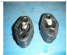
Install rubber isolators from Step 2 onto hitch with M12 hex bolts. Secure the isolators with M12 flat washers and nylock hex nuts as shown.
