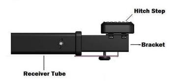
WARNING- iBoard<sup>™</sup> Hitch Step may Interfere with the operation of the O.E. back-up sensor on several late model vehicles. If your vehicle comes equipped with an O.E. back-up sensor, it is advised that you check its' functionality after installation.
