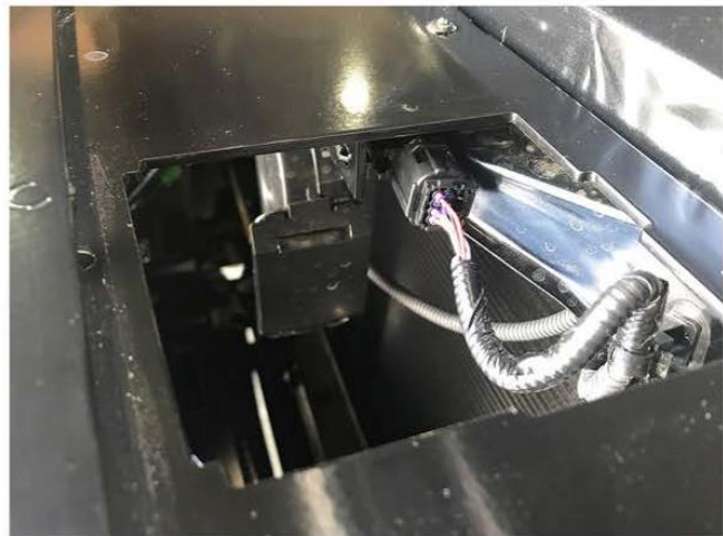
10. Install grille to vehicle. Connect TSS harness.
