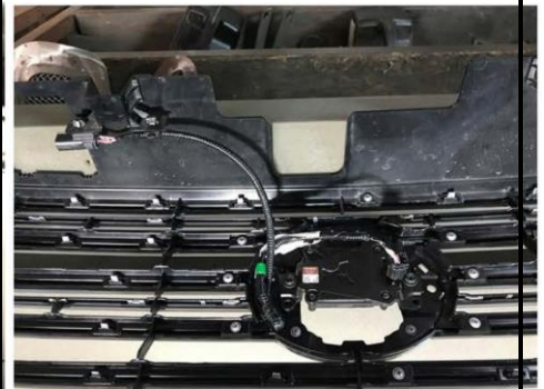
3. Remove TSS sensor module and harness from factory grille. Note the TOP side orientation of the sensor.
