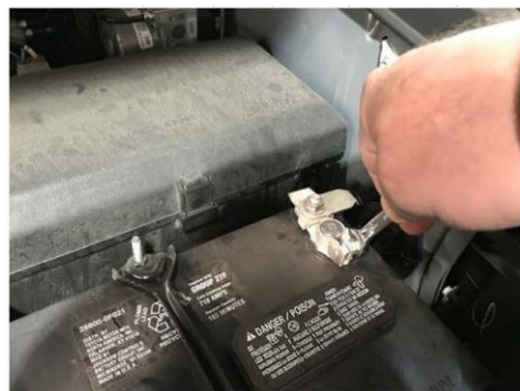
1. Disconnect negative battery terminal.
