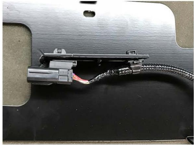
8. Press harness cable mounts into bracket as shown.
