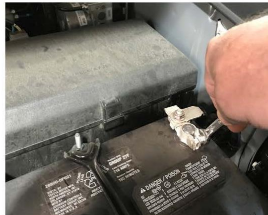
12. Reconnect negative battery terminal.
