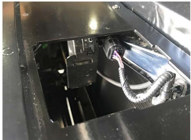
10. Install grille to vehicle. Connect TSS harness.
