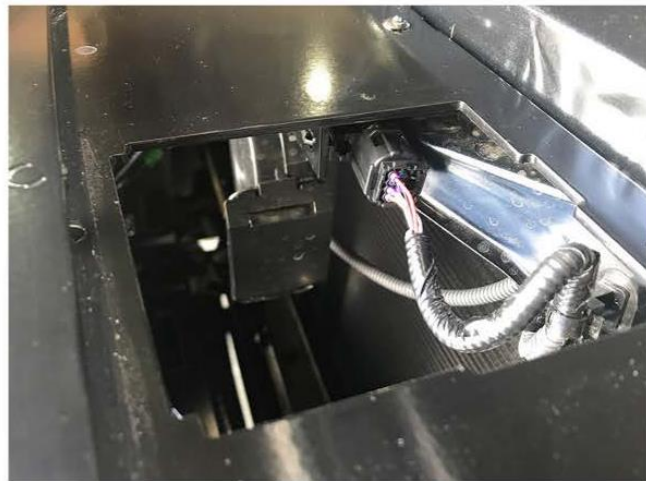
10. Install grille to vehicle. Connect TSS harness.
