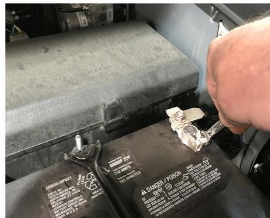
12. Reconnect negative battery terminal.
