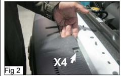
3. Remove four 10mm bolts from the plastic radiator cover then remove the
