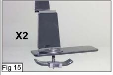
**17**. Take the two flange brackets (with the u-nuts installed)and attach them onto the large ends of the bottom extension brackets with one #8X3/4" screw and one 1" black fender washer. You will only need to screw the threads in a couple of turns as you want the flange brackets to have some space between them and the bottom extension bracket (Fig 15). You will have two assembled bottom extension brackets.
