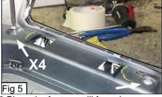
6.Place the factory grill face down on a clean soft surface (take special care to protect the chrome factory shell). On the back of the grille assembly use a Phillips screwdriver to remove two Phillips screws from each side of the factory grille (4total) (Fig 5).
