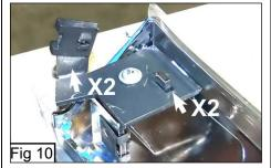
12. Take the two top plate extension brackets and install them on the upper corners of the factory grille shell using the factory screws to secure them to the grille shell (Fig 10) and install the u-nuts onto the arms of the brackets as shown in (Fig 10). Insure the u-nut is oriented with the side that accepts the screw facing outward as shown.
