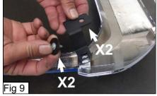
from the factory grille by pressing the 11. Take the two Z support brackets tabs on the back of the logo inward and install them on backside of the factory grille shell with the arm bending downward as shown (Fig 9). Use the factory screws removed in Step 4 along with one I" black fender washer on each bracket to secure the bracket to the factory grille shell. Repeat this on the opposite side of the factory grille. Tighten the two screws
