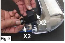
11. Take the two Z support brackets and install them on backside of the factory grille shell with the arm bending downward as shown (Fig 9). Use the factory screws removed in Step 4 along with one I" black fender washer on each bracket to secure the bracket to the factory grille shell. Repeat this on the opposite side of the factory grille. Tighten the two screws
