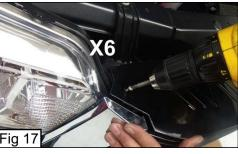
19. Take the billet grille and place it into 20. Insert two #10 screws through the chrome factory grille shell. Take six #10 screws and secure the top plate to the vehicle by inserting the screws through the six holes in the top plate and tighten (Fig 17).
