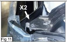
13. Reinstall the factory chrome grille shell (with the brackets installed) on the vehicle, make sure the brackets slide under the black plastic arms on the core support (Fig 11) and that the holes in the u-nut and bracket line up with the hole in the plastic bracket on the core from (Fig 12). Make sure the fastener support.
