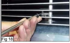
the billet bars at the bottom of the billet grille, through the mounting plates with holes in them on the back of the Billet and into the bottom extension brackets and tighten (Fig. 18).
