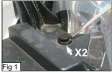
2.From underneath the hood remove two plastic fasteners from the factory grille located near the headlamps radiator cover (Fig 2). with a flat screwdriver (Fig 1).
