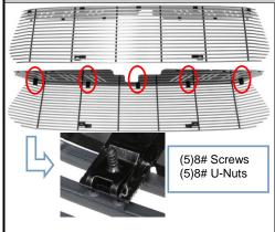
1. Identify the grille & hardware with parts list. Install Billet Grille and back plate with 5 screws and 5 U-Nuts.
