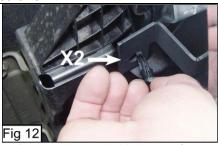
14.Reach down behind the factory grille and locate the brackets that you installed on step 7 and insert the factory plastic fastener through the hole in the bracket and into the same hole in the vehicle it was removed is fully inserted and secure.
