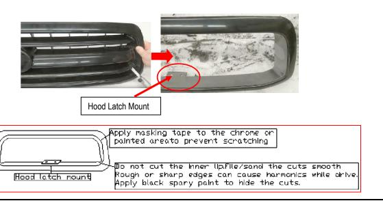
The instruction here is for your reference only. You may need to bend the billet grille bars or tabs a little bit to adjust to fit. We strongly recommend the professional installer for best result.
