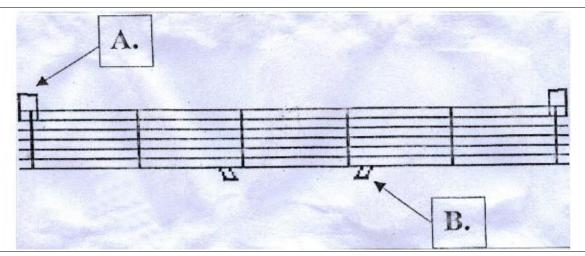
4 Close the hood and check the alignment of the billet insert. If necessary, remove the insert and adjust the brackets.
