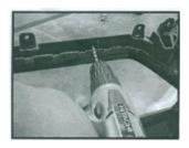
16. Drill a 3/16 inch holes for the mounting screws.
