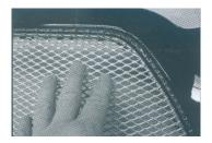
14. Place the mesh grille insert into the factory grille shell from the front side as shown.
