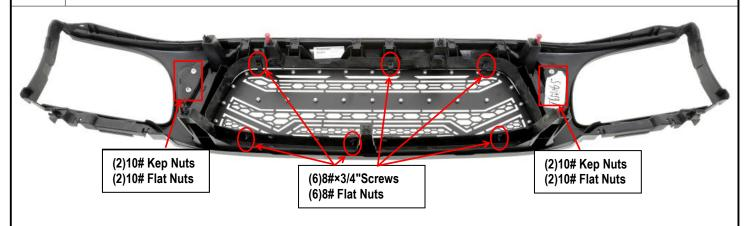
The instruction here is for your reference only. You may need to bend the billet grille bars or tabs a little bit to adjust to fit. We strongly recommend the professional installer for best result.
