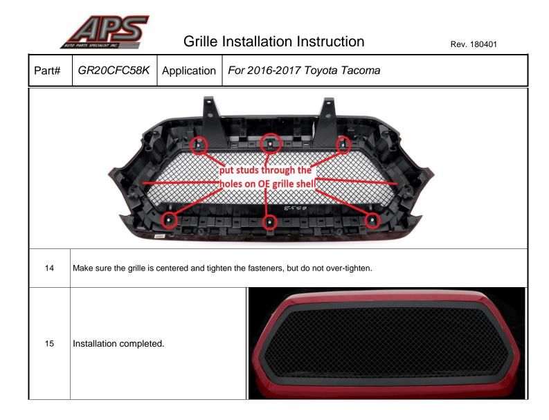
The instruction here is for your reference only. You may need to bend the grille a little bit to adjust to fit. We strongly recommend the professional installer for best result. We are not responsible for any damage caused by the installation. Thank you for choosing our product!
