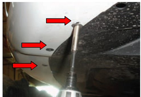
Step 2-4: Remove 7 Screws from Underneath of the Factory Front Bumper
