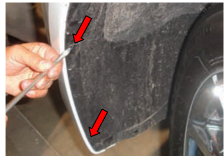
Step2-2: Remove 2 clips on side Fender Well
