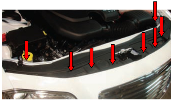
Step 2-1: Pop hood. Remove 8 clips on the Plastic Cover
