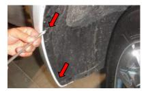
Step2-2: Remove 2 clips on side fender well
