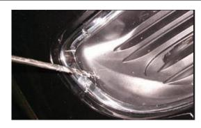
Step3-3: Drill a 3/16 Hole where you marked the Screws.
