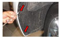
Step2-2: Remove 2 clips on side fender well
