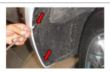
Step2-2: Remove 2 clips on side fender well
